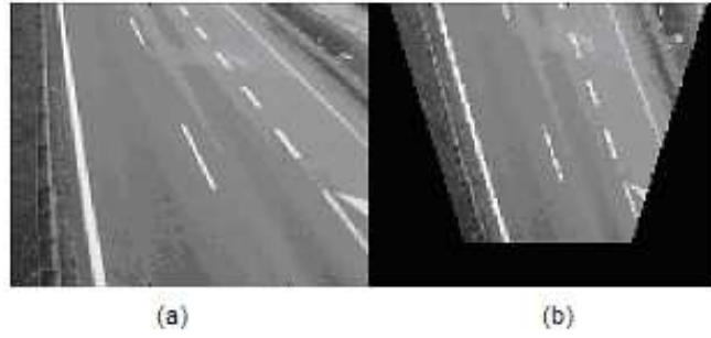
Fig. 12 Example of original image (a) and result of transformation (b) for \varphi=43^\circ , h=15\text{m} , f=2.8\text{mm} using the reverse of (22) and (23)
