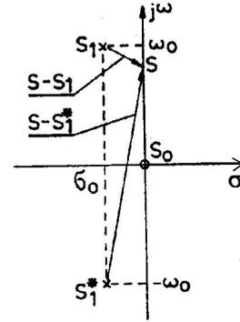
Fig. 7. Location of the vectors:  $|s - s_0|$ ,  $|s - s_1|$ ,  $|s - s_1^*|$  as a function of  $s = j\omega$  for the impedance  $Z(s)$ .
