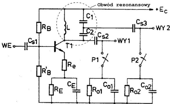
Fig. 2. Amplifier with a single parallel resonance circuit.
