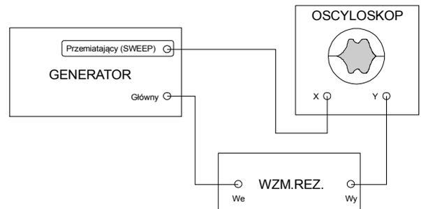
Fig.1. Amplifier with a single parallel resonance circuit - measurement arrangement.
