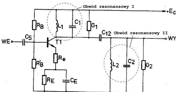
Fig. 11. Amplifier with a pair of LC resonant circuits
