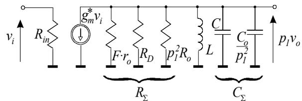
Fig. 5. Equivalent circuit of the amplifier with a single resonant circuit, taking into account certain parameters of the transistor, the dynamic resistance of the coil, and the load.
