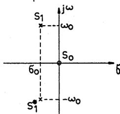
Fig. 6. Distribution of zeros and poles of the impedance  $Z(s)$ .
