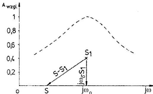
Fig. 10. Geometrical determination of the resonance curve of the amplifier with a single resonant circuit.
