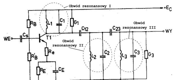
Fig. 14. Amplifier with a triple resonant circuit coupled capacitively
