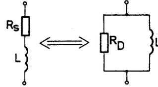
Fig. 4. Equivalence between the winding resistance and the dynamic resistance of the coil.
