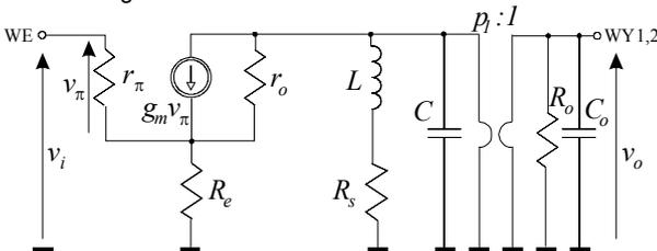
Fig. 3. Small-signal equivalent circuit of the amplifier of Fig. 2
