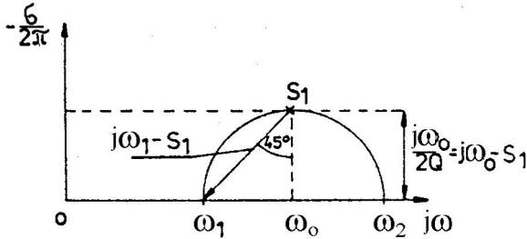
Fig. 9. Determination of the 3-dB amplifier bandwidth.
