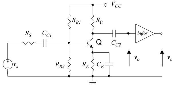
Fig. 2. Amplifier configuration diagram of a common-emitter (CE).
