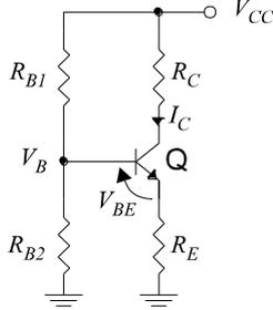
Fig. 3. The circuit diagram for counting of the operating point.
