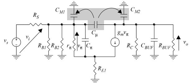
Fig. 9. Substitute small signal diagram of the amplifier in a CE-RE shown in Fig. 7 to determine the upper cut-off frequency.
