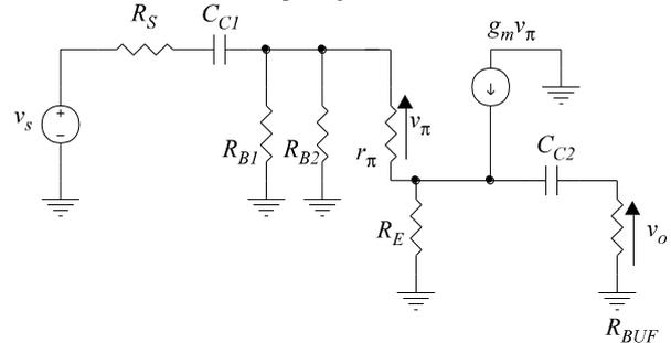
Fig. 14. A substitute small signal scheme of the amplifier circuit CC shown in Fig. 11 to determine the lower cut-off frequency.
