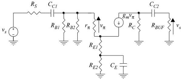
Fig. 10. A substitute small signal scheme of the amplifier in a CE-RE shown in Fig. 7 to determine the lower cut-off frequency.
