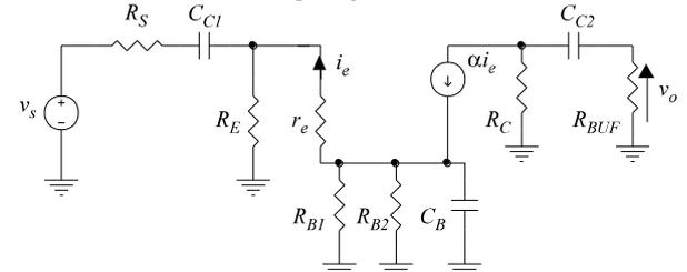
Fig. 18. A substitute small signal scheme of the amplifier circuit CB shown in Fig. 15 to determine the lower cut-off frequency.
