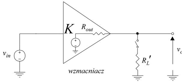
**Fig. 20. Method for measurement of output resistance of the amplifier.** Marking as well  $v_o$  as  $v_o'$  respectively output voltages at the opened and bypassed resistor get:
