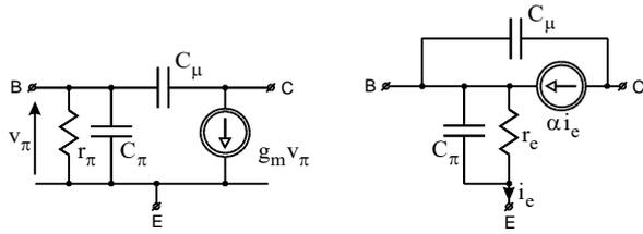
Fig. 1. Small Signal circuit substitute π type and T-type of the bipolar transistor.
