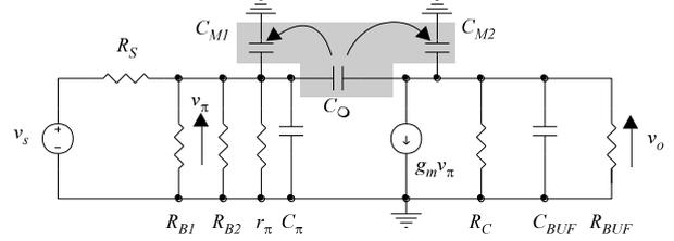
Fig. 5. A substitute small signal scheme of the amplifier in a CE of Fig. 2 to determine the upper cut-off frequency
