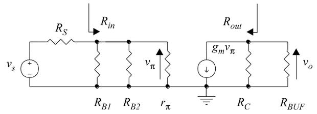
Fig. 4. A substitute small signal scheme of the amplifier in a CE of Fig. 2 for the medium frequency range.
