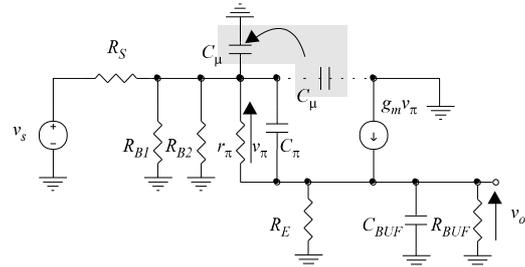
Fig. 13. A substitute small signal scheme of the amplifier circuit CC shown in Fig. 11 to determine the upper cut-off frequency.
