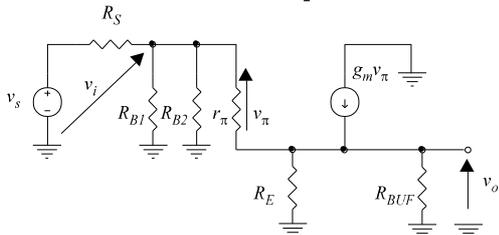
Fig. 12. A substitute small signal scheme of the amplifier circuit CC shown in Fig. 11 for the medium frequency range.
