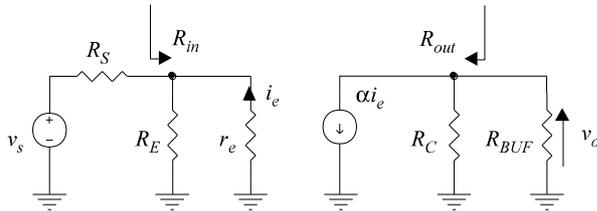
Fig. 16. A substitute small signal scheme of the amplifier circuit CB shown in Fig. 15 for the medium frequency range.
