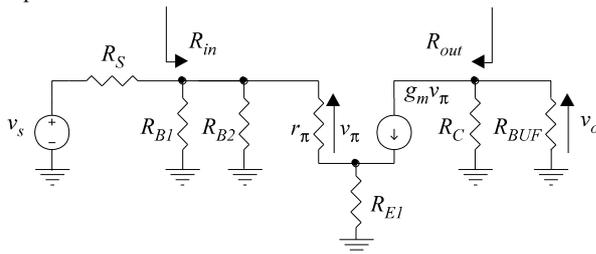
Fig. 8. The substitute small signal scheme of the amplifier in a CE-RE shown in Fig. 7 for the medium frequency range.
