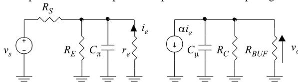
Fig. 17. A substitute small signal scheme of the amplifier circuit CB shown in Fig. 15 to determine the upper cut-off frequency.
