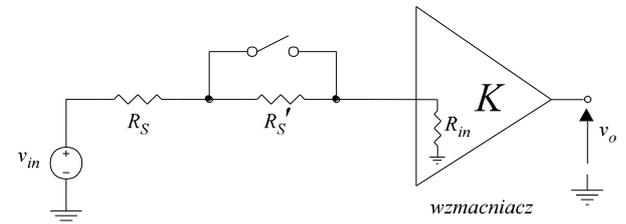
Fig. 19. Method for measurement of input resistance of the amplifier.
