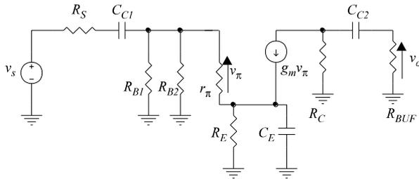
Fig. 6. A substitute small signal scheme of the amplifier in a CE of Fig. 2 to determine the lower cut-off frequency
