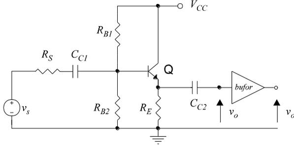
Fig. 11. The configuration diagram of the amplifier in the common collector (CC).
