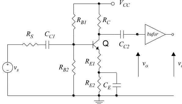
Fig. 7. Amplifier configuration diagram of a common-emitter with not bypassed resistance  $R_{E1}$  (CE-RE).
