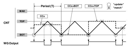
The dual-slope PWM result in a lower operating frequency at equal resolution compared to the single-slope PWM mode.
