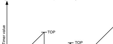
Figure 3-2. Normal mode with period setting.
