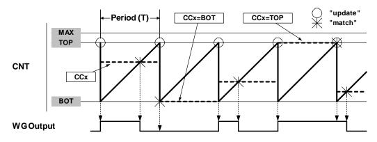
The single-slope Pulse Width Modulation (PWM) provides twice the PWM frequency compared to dual-slope PWM. The high frequency makes this mode well suited for power regulation, rectification, and DAC applications. High frequency allows physically small sized external filtering components, which reduces total system cost.
