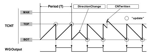
The waveform generated will have a maximum frequency of  $f_{clk}/2$  when CCA[H:L] is set to zero (0x0000). The waveform frequency is defined by Equation 3-1.
