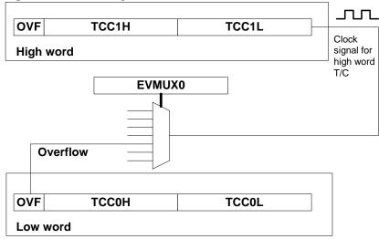
Figure 5-1. Cascading two 16-bit Timer/Counter modules.
