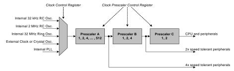
The default setup after a reset is to select the internal 2 MHz RC oscillator and pass the clock signal undivided through all three prescalers. Prescaler A can be used to
