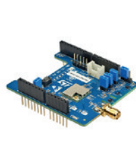
EXPANSION BOARD P/N: I-NUCLEO-LRWAN1 (ST and USI®)
