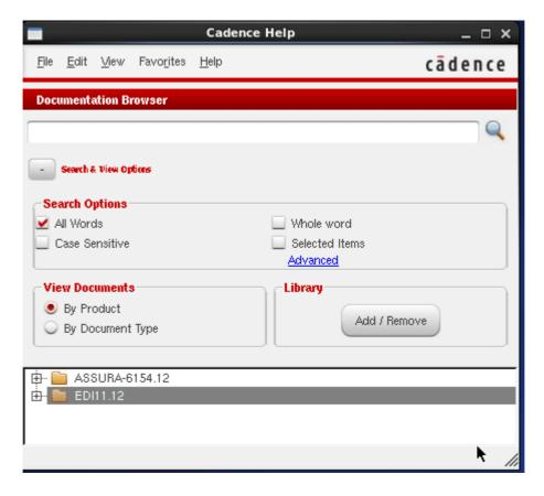
There are possible help packets to be selected at the bottom of the **Cadence Help** window. In the above figure it is **ASSURA-6154.12** and **EDI11.12**. To add other necessary packets click button **Add/Remove** in the **Library** subwindow and next press **Add**. and then from the list of the available can be chosen needed one, please observe example explaining help packets location below:
