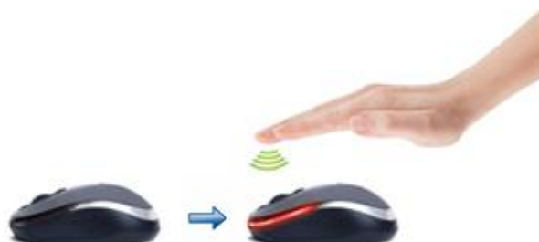
Figure 2-43. Wake-on-Approach Implemented in a Mouse
