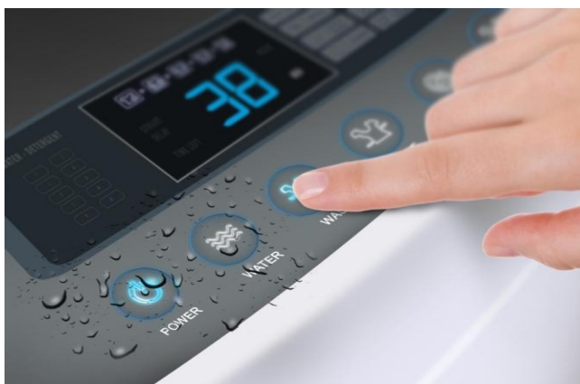
Figure 2-31. CapSense-based Touch User Interface in a Washing Machine with Liquid Tolerance
