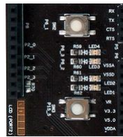
Figure 4: SW2 (pin P6_1) and SW3 (pin P15_5)
