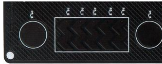
Figure 3: CapSense Buttons (pin P5_5 and P5_6) and Slider (pins P5_0..P5_4)
